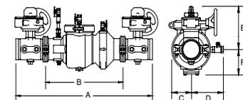
Attention: Model 350A (grooved body) & Model 350 (flange body) have different lay lengths.
