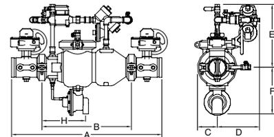
Attention: Model 375ADA (grooved body) and Model 375DA (flange body) have different lay lengths.
