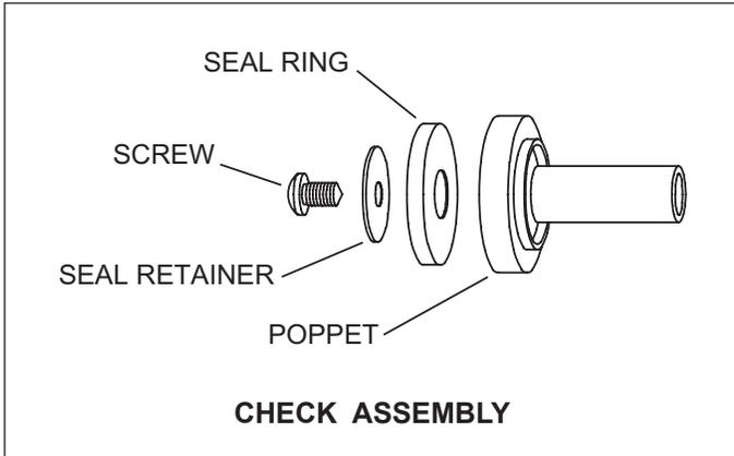
All Model 950XLT2 Double Check Valve Backflow Preventers must be inspected and maintained by licensed personnel at least once a year or more frequently as specified by local codes. Replacement of worn or damaged parts must only be made with genuine "ZURN WILKINS" parts.
