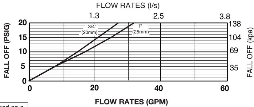
"Flow curves are based on a 50 psi pressure differential"
