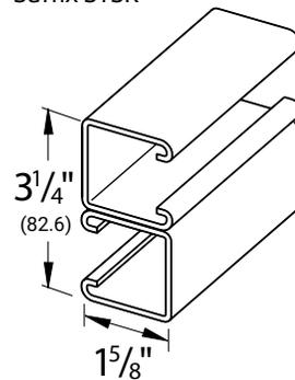
Our welded channels are spot welded 2" (50.8mm) on center, dimensions shown are for welded variations of any channel with or without slotted holes.
