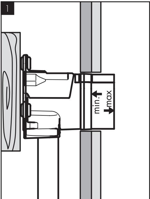
This valve should be attached to a header using screws (not included).
