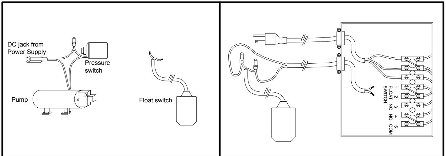
**Step 3:** Complete MF200 circuit without float switch.
