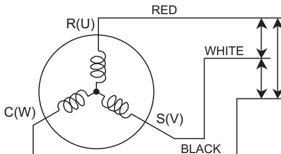
→ If the resistance value is 0  $\Omega$  or infinite, replace compressor.
