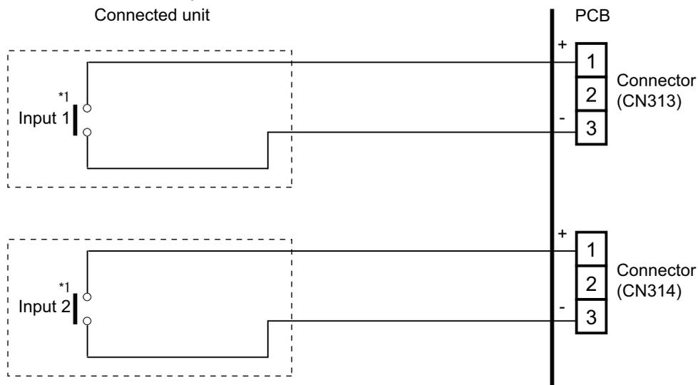
\*1: The switches can be used on the following condition: DC 12 V to 24 V, 1 mA to 15 mA.
