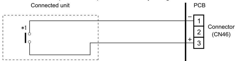
\*1: The switch can be used on the following condition: DC 12 V to 24 V, 1 mA to 15 mA.
