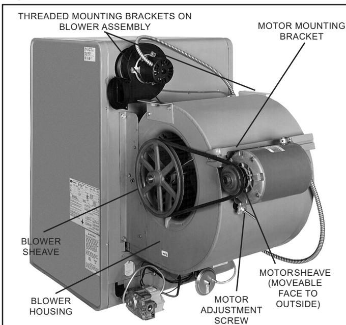
3. Adjust motor adjusting screw for a belt deflection of approximately 3/4" with five pounds of force applied midway between the sheaves (see Figure 14.3). Since the belt tension will decrease dramatically after an initial run-in period, it is necessary to periodically re-check the tension. Excessive tension will cause bearing wear and noise.
