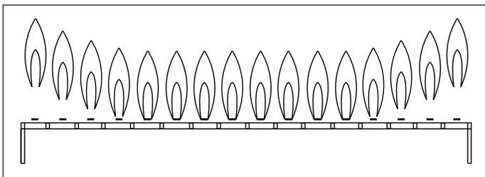
**Figure 28.3 - Floating Flame Condition**
