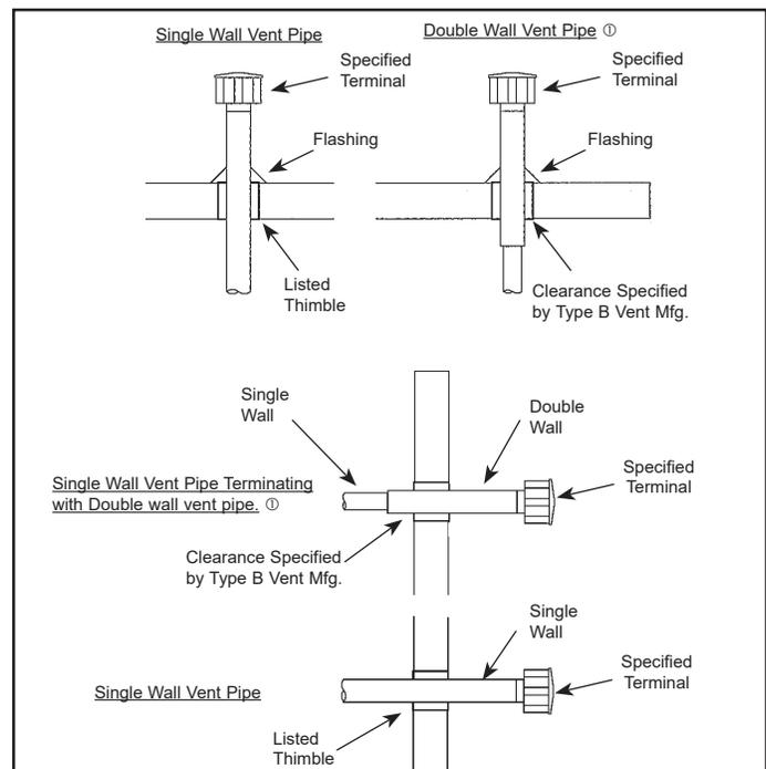
① See Instruction A12 for attaching single wall pipe to double wall pipe.
