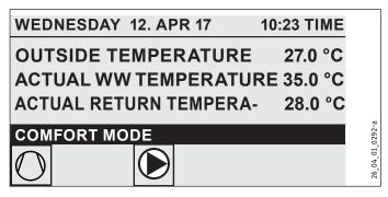
If you want to select another operating mode, use the Touch-Wheel. This takes you through the list of possible operating modes. The current choice (list entry) is shown in the shaded selection field. Setting the WPM to Programmed Operation will allow for scheduling between the Comfort and Eco temperature setpoints at different times and days of the week.
