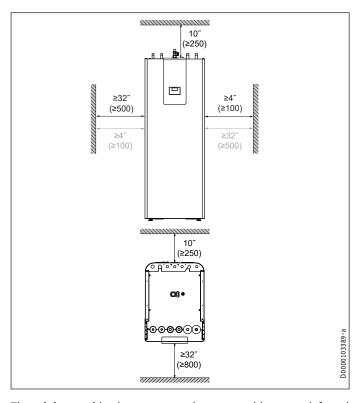
The minimum side clearances can be swapped between left and right.
