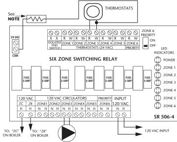
**Operation:** When any thermostat calls for heat, the boiler is given a signal to start. The appropriate circulator is energized only when the boiler temperature is above the set low limit.
