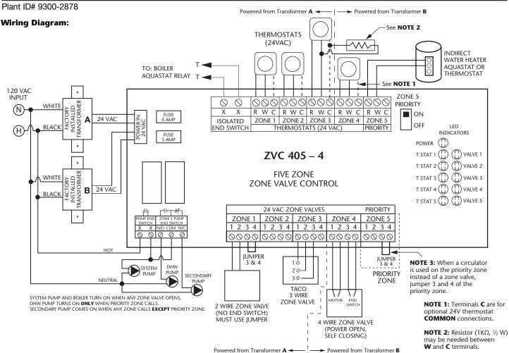
**Operation/External Diagnostics:** When any thermostat calls for heat, the appropriate zone valve is energized and the yellow light goes on. When the zone valve is fully open, the red light goes on and energizes the end switch relay. The green light should always be on, indicating that power is connected.
