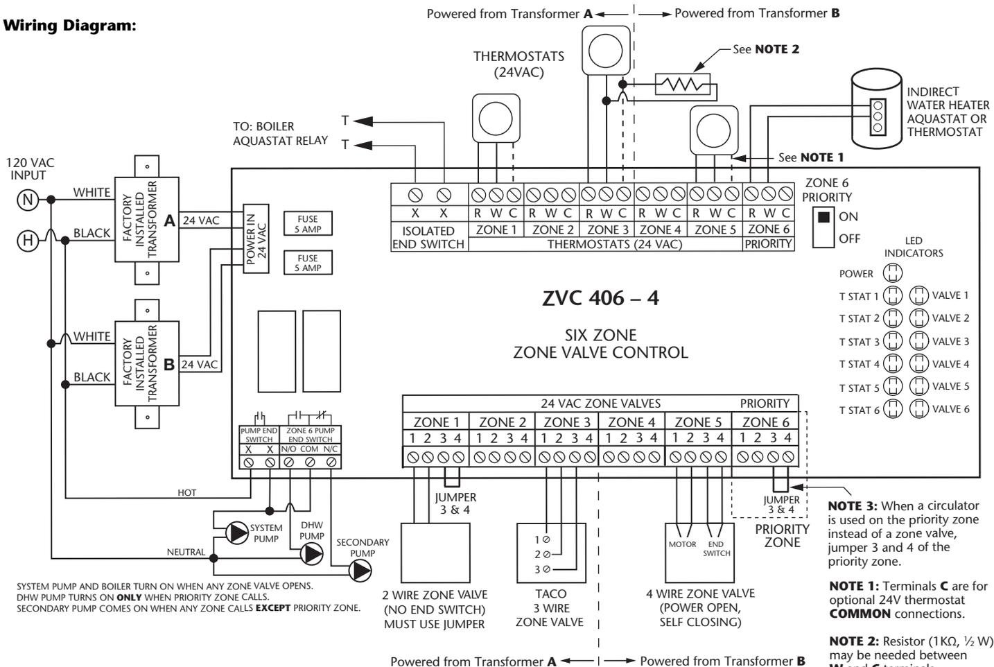
**Operation/External Diagnostics:** When any thermostat calls for heat, the appropriate zone valve is energized and the yellow light goes on. When the zone valve is fully open, the red light goes on and energizes the end switch relay. The green light should always be on, indicating that power is connected.
