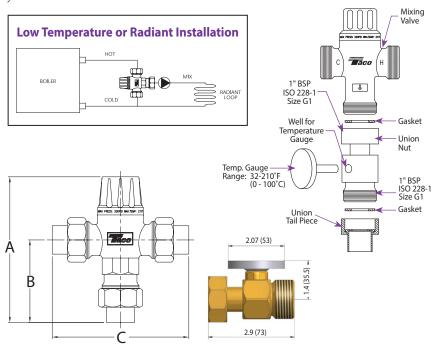
**5000 Series Heating Only Mixing Valve Dimensions** Dimensions for reference only
