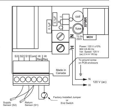
Do not run the wires parallel to telephone or power cables. If the sensor wires are located in an area with strong sources of electromagnetic interference (EMI), shielded cable or twisted pair should be used or the wires can be run in a grounded metal conduit. If using shielded cable, the shield wire should be connected to the Com terminal on the PC Board and not to earth ground.
