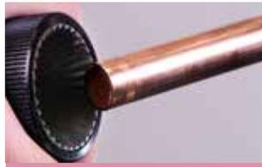
**2. Deburr and remove all external sharp edges**
