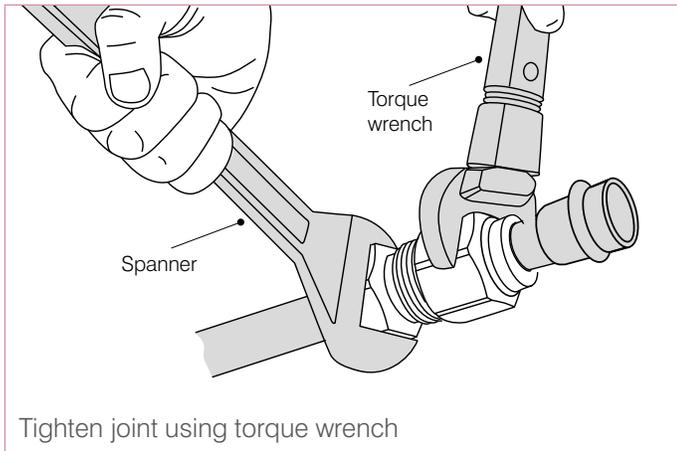
Fully tighten using spanner and torque wrench to the torque values set out in table 8. **Do not over tighten.**
