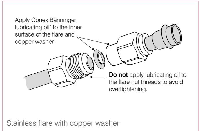
Align the centers of both flares and tighten the flares by hand.
