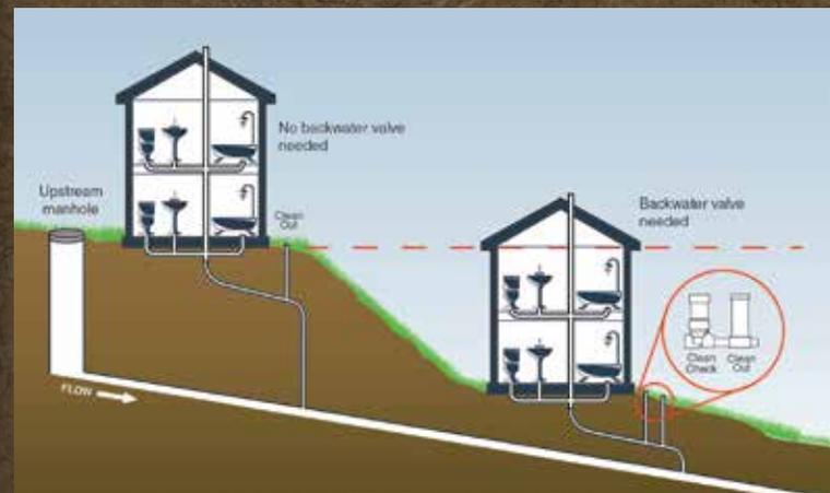
Waste water flow from structure. (Flapper opens)
