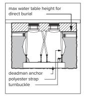
buried in high water table scenarios must be installed with an anti-flotation anchor kit. Models GB-50, GB-75, and GB-250 use model AK1 anchor kit. Model GB-500 uses model AK2 anchor kit for use with deadmen anchors. Models GB-1000, GB-1500, GGI-750 and GGI-2000 use model AK3 anchor kit for use with deadmen anchors
