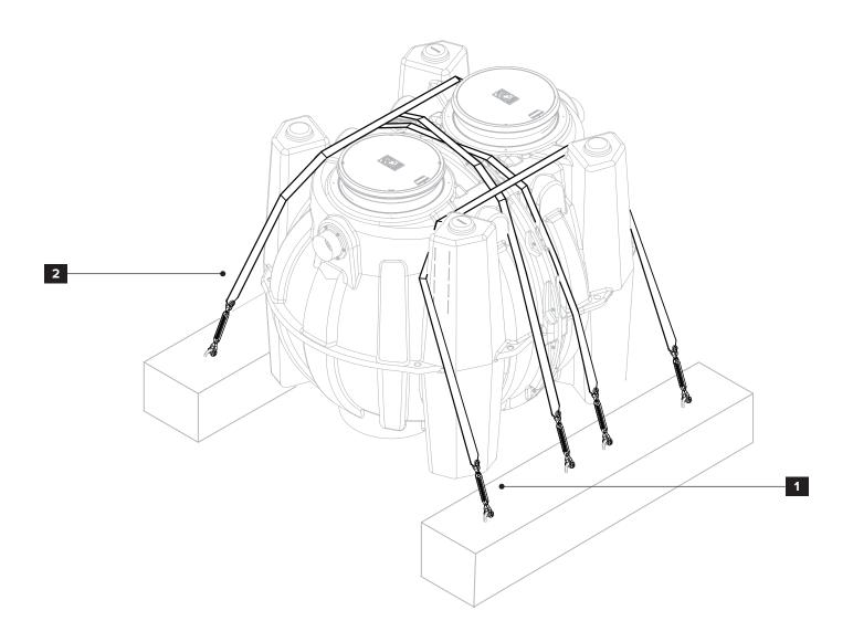
**1.** Jaw-Jaw Galvanized Turnbuckle (x8)
