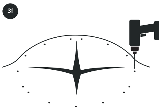
Drill (or cut) holes in the membrane for the Lag Screws. Take care not to drill out the threaded holes for the Lag Screws in the Mounting Ring.
