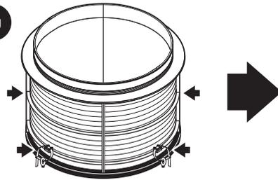
Loop cable ties through mounting holes and eyebolts, do not tighten.
