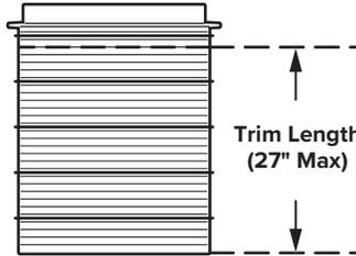
**1c** Measuring from bottom of riser, mark trim length and cut riser halves.
