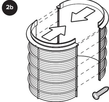
Immediately assemble riser halves after applying sealant and fasten using supplied screws.
