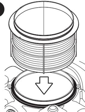
Place riser into position aligning vertical ribs with eyebolts.
