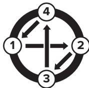
Tighten cable ties, a little bit at a time in a star pattern going around the riser to evenly force the riser into the mastic sealant. Riser should go 1/2" - 3/4" into the sealant.
