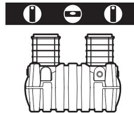
Make final adjustments to cable ties to ensure riser is level.
