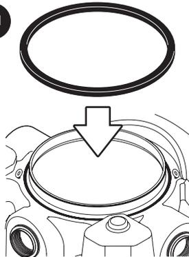
Lay butyl mastic sealant into the channel surrounding the accessway.
