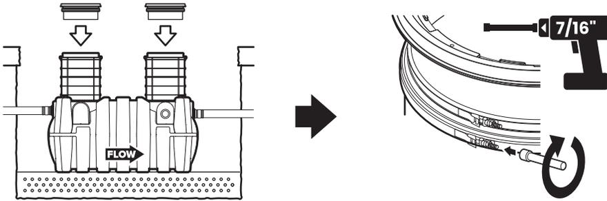
Place cover adapter/gasket assembly onto top level riser(s). Tighten lower band clamp to 5 -8 ft. lbs. of torque using 7/16" nut driver bit.
