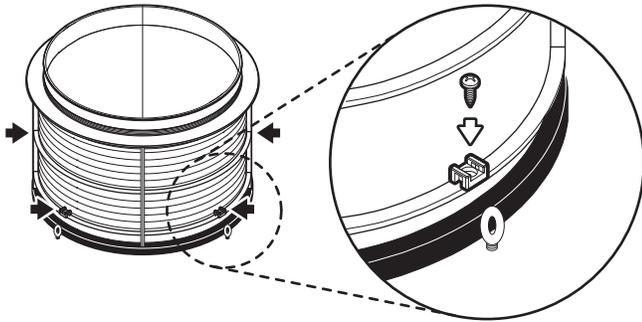
Install 4 cable tie mounts onto lowest horizontal structural rib using #10 x 3/4" screws. Make sure mounts are located directly above eyebolts and are positioned for horizontal cable tie placement.
