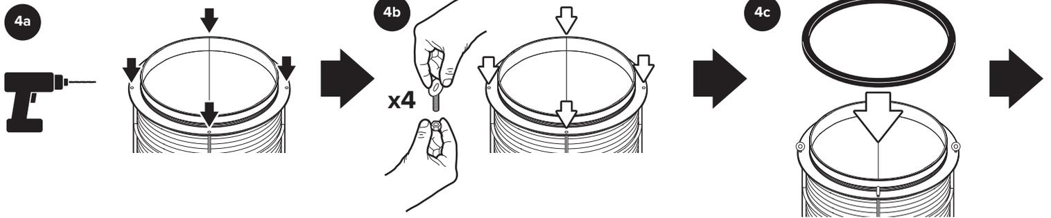
On bottom riser: drill (4) 1/4" mounting holes through flange.
