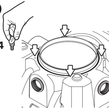
Remove insert plugs, then hand tighten eyebolts into threaded holes surrounding the accessway.
