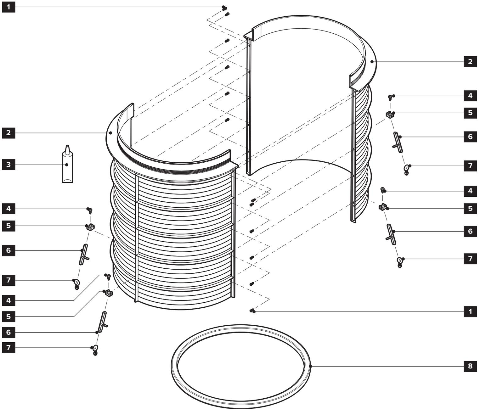
1. #8 x 5/8" riser body assembly screw (x12)
