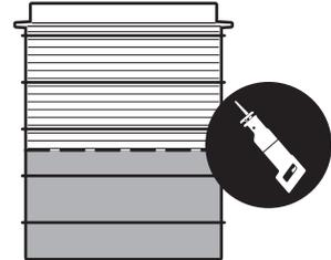
**NOTE:** If trim length is 0 or less, no cutting is required. Trimming risers using these guidelines will result in risers that are 0-2" shorter than the exact riser height needed. Cover Adapter adjustability will allow for final adjustments to grade.
