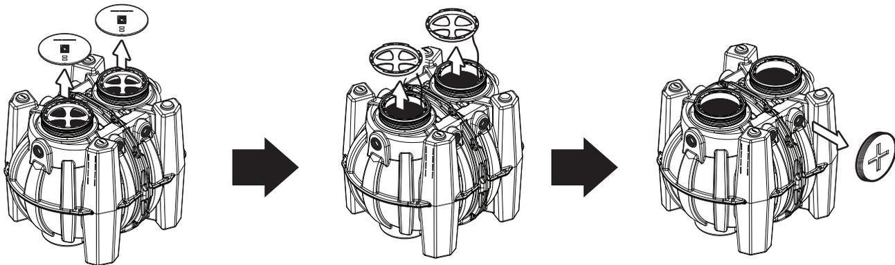
Remove cover bolts (if applicable), then remove covers. Remove Safety Star® inserts, leave tethered to unit. Install cleanout plugs to two unused pumpout port connections.
