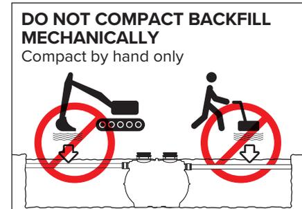
Fill unit with water for stabilization and float-out prevention. Backfill evenly around tank using crushed aggregate (approximately 3/4" size rock or sand with no fines) or flowable fill. **Do not mechanically compact backfill around unit.**
