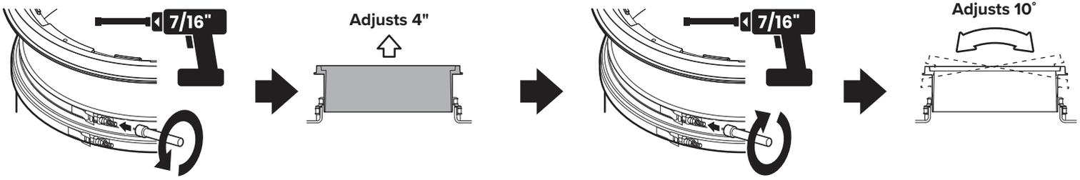
Loosen the cover adapter upper band clamp using 7/16" nut driver bit. Adjust cover adapter heights as needed. **Maintain a minimum 2-1/2" insertion depth.** Tighten upper band clamp to 5-8 ft. lbs. of torque using 7/16" nut driver bit. If required, cover adapters may now be tilted up to 10° in any direction using gasket flexibility.
