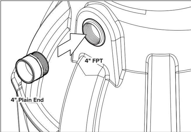
Screw plain end fittings (included) into bulkhead fittings using pipe thread sealant or tape approved for use with plastics. 6" connection types come pre-installed from the factory.
