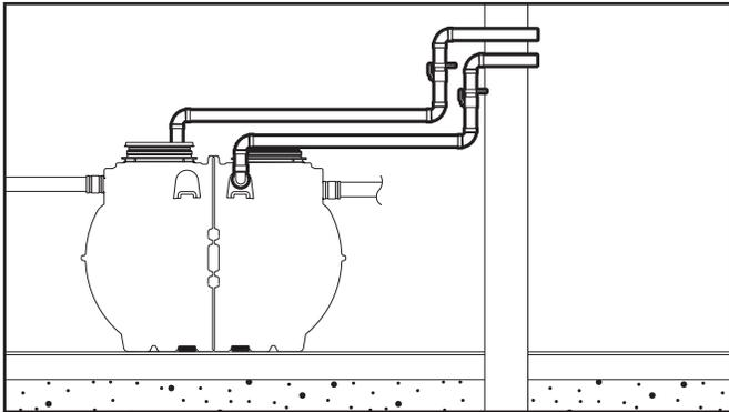
Install 3" PVC piping, connections, valves and/or hardware from the interceptor pumpout port to pumpout hook-up location (**Not included with this unit**). Maximum quantity of 6 elbow fittings. Max. height from static water line of interceptor to hook-up is 21 feet. Max horizontal distance from interceptor to pumper truck (including hose) is 100 feet.
