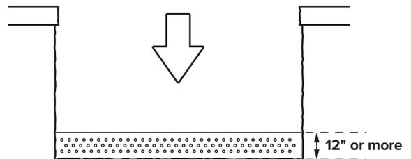
Excavate hole at least 18" larger than interceptor on all sides and 12" deeper than tank bottom. Lay a level bed of well-packed, crushed aggregate (approximately 3/4" size rock or sand, with no fines) in the base of hole.
