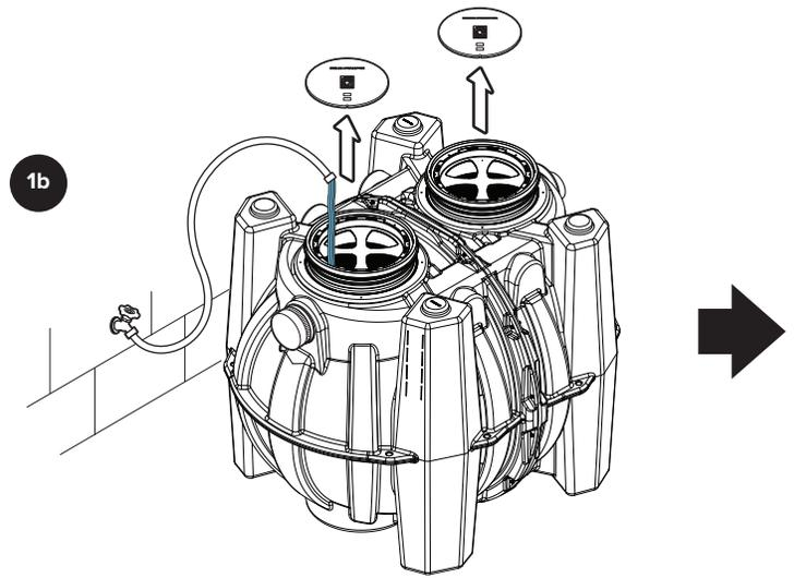
Remove covers. For base unit testing fill with water to just above the highest connection.
