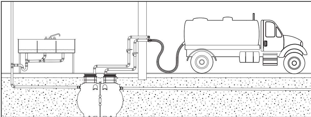
Run sinks to ensure interceptor is full of water. Attach pumper hose to 3" cam and groove fitting. Turn on pump, make sure interceptor is pumped out and inspect pumpout plumbing for leaks.
