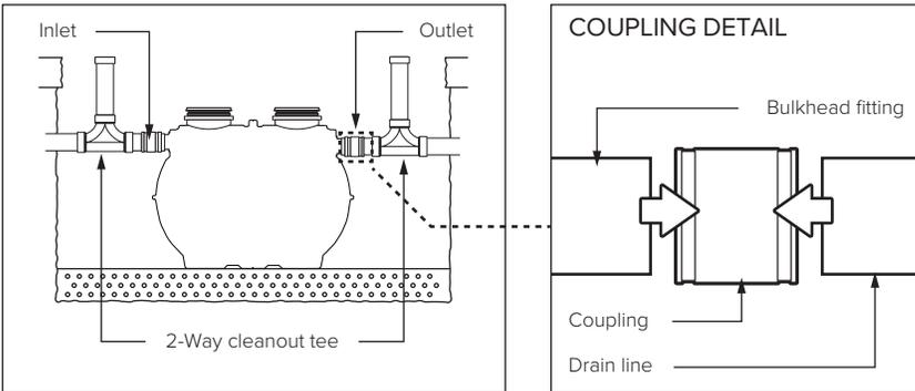
Place unit into final position and set level. Mechanically couple inlet and outlet drainage lines to unit. **Do not solvent weld.** Ensure all upstream fixtures are trapped. Vent per local code. Installation of 2-way cleanout tees to grade (by others) is recommended for buried installations.
