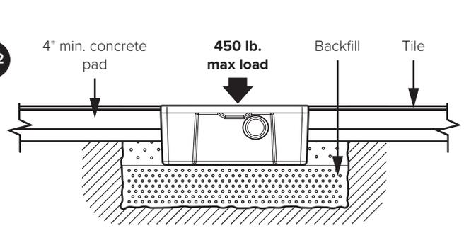
**Flush-to-Grade Burials:** Not recommended for heavy foot traffic areas. Backfill evenly around tank using crushed aggregate (approximately 3/4" size rock or sand, with no fines), finish with a minimum 4" thick concrete pad.
