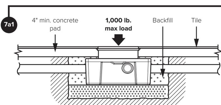
**Below Grade with Riser (preferred):** See instructions included with FCR1 riser. Backfill evenly around tank using crushed aggregate (approximately 3/4" size rock or sand, with no fines), finish with a minimum 4" thick concrete pad.
