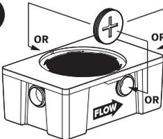
Cap all unused connection points with 4" cleanout plugs using pipe thread sealant or tape approved for use with plastics.
