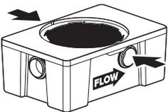
**2b** Unscrew diffuser retaining nut and remove outlet diffuser.
