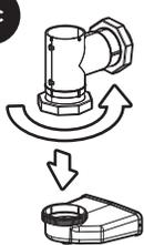
**2d** Rotate diffuser toward chosen outlet, replace foot ensuring it will point to the back wall of the unit and hand tighten foot retaining nut.
