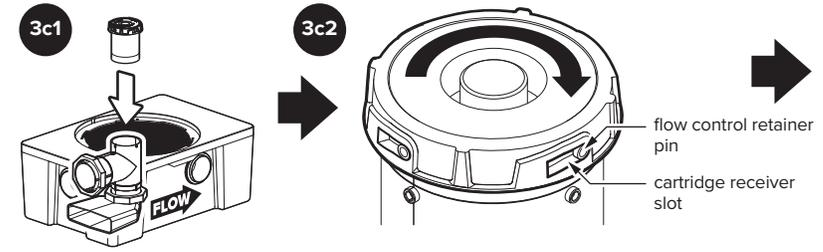
Slide flow control cartridge into top of inlet diffuser and rotate clockwise until cartridge drops onto flow control retainer pins. Continue rotating clockwise until PVC primer/cement are fully seated.
