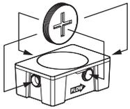
**1b** Remove cover and fill with water to just above the highest connection. For riser system testing (if required) fill to finished grade level. **CAUTION:** Support risers before filling to prevent tipping. Inspect unit, connections and gaskets for leaks. Check water level at specific time intervals per local code.
