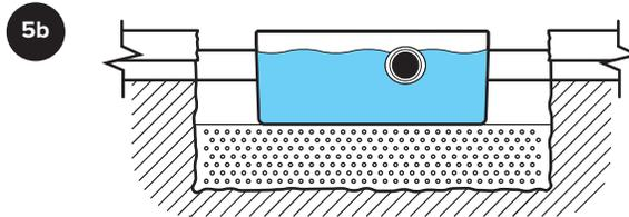
Set interceptor and connect piping using pipe thread sealant or tape approved for use with plastics. **Vent per local code.** Fill tank with water so that it remains in place during backfill.
