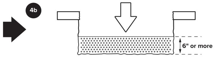
Add crushed aggregate (approximately 3/4" size rock or sand, with no fines) to base of hole.
