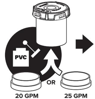
Rotate flow control cartridge counter-clockwise to release and remove from inlet diffuser
