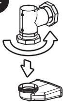
**2d** Rotate diffuser toward chosen outlet, replace foot ensuring it will point to the back wall of the unit and hand tighten foot retaining nut.
