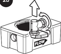
**2c** Unscrew diffuser foot retaining nut and remove outlet diffuser foot.
