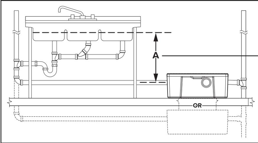
**Note to Plumbing Inspector** This interceptor includes certified internal flow control and does not require a dedicated “Flow Control Vent” (air intake).
