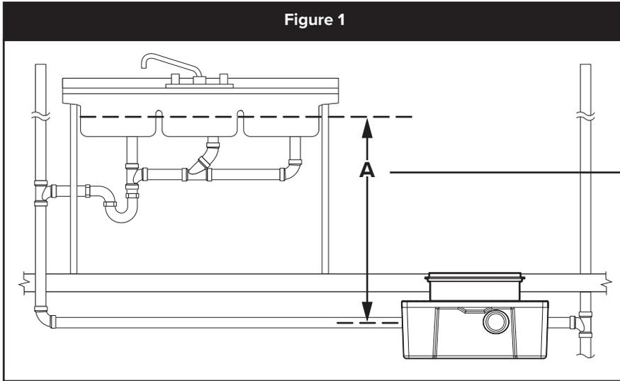
**Note to Plumbing Inspector** This interceptor includes certified internal flow control and does not require a dedicated "Flow Control Vent" (air intake).
