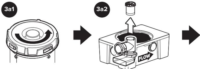
Rotate flow control cartridge counter-clockwise to release and remove from inlet diffuser
