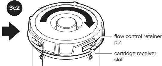
Slide flow control cartridge into top of inlet diffuser and rotate clockwise until cartridge drops onto flow control retainer pins. Continue rotating clockwise until pins are fully seated.
