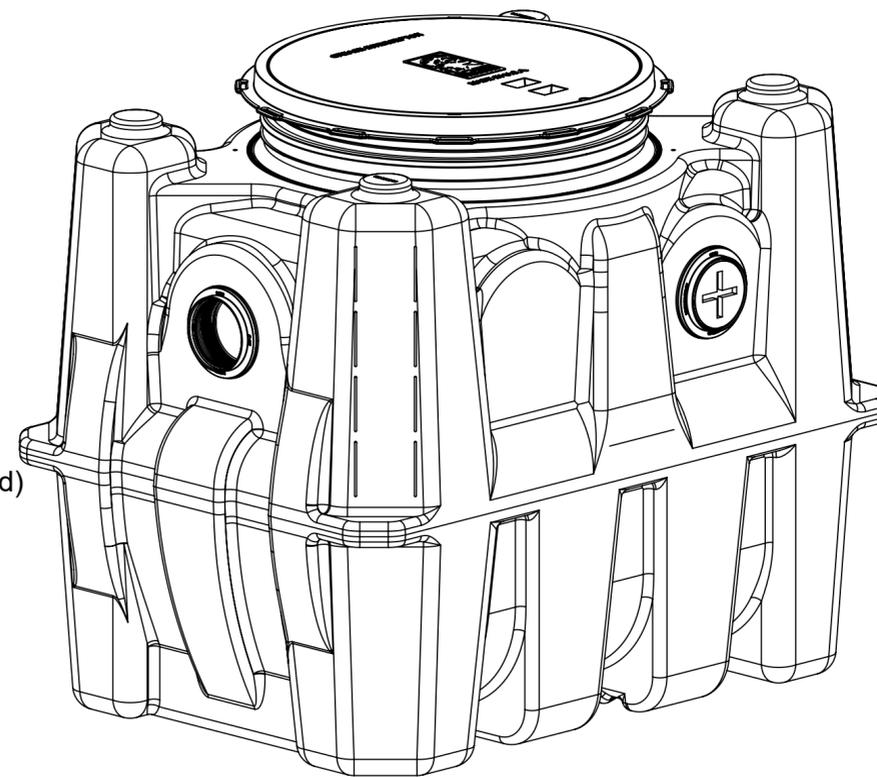
Adjustable Adapter with H-20 rated cast iron cover
