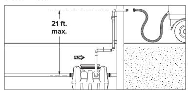
Plumbing from interceptor to hook-up to have a maximum quantity of 6 elbow fittings.
