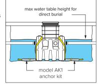
direct buried in high water table scenarios must be installed with an anchor kit. Model GB-75 uses model AK1 anchor kit.
