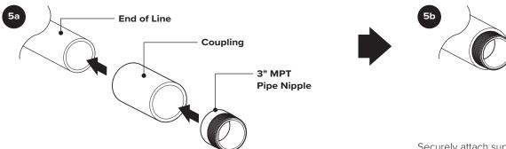
At the end of the pumpout plumbing line, install a 3" MPT pipe nipple (**Not included with this kit**) using a coupling of your choice.
