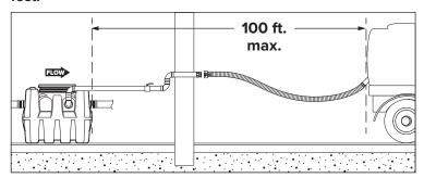
Maximum vertical distance from static water line of grease interceptor to pumpout port hook-up shall not exceed 21 feet.
