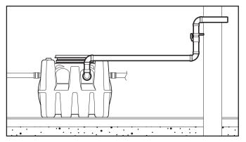
Install 3" or 2" PVC piping, connections, valves and/or hardware from the interceptor pumpout port to pumpout hook-up location (**Not included with this kit**). Maximum quantity of 6 elbow fittings. Max. height from static water line of interceptor to hook-up is 21 feet. Max horizontal distance from interceptor to pumper truck (including hose) is 100 feet.
