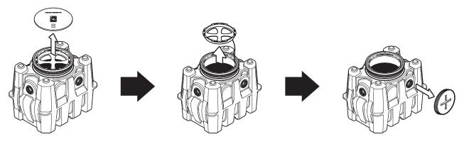
Remove cover bolts (if applicable), then remove cover. Remove safety star insert, leave tethered to unit. Remove preinstalled cleanout plug from outlet chosen to become a pumpout port.
