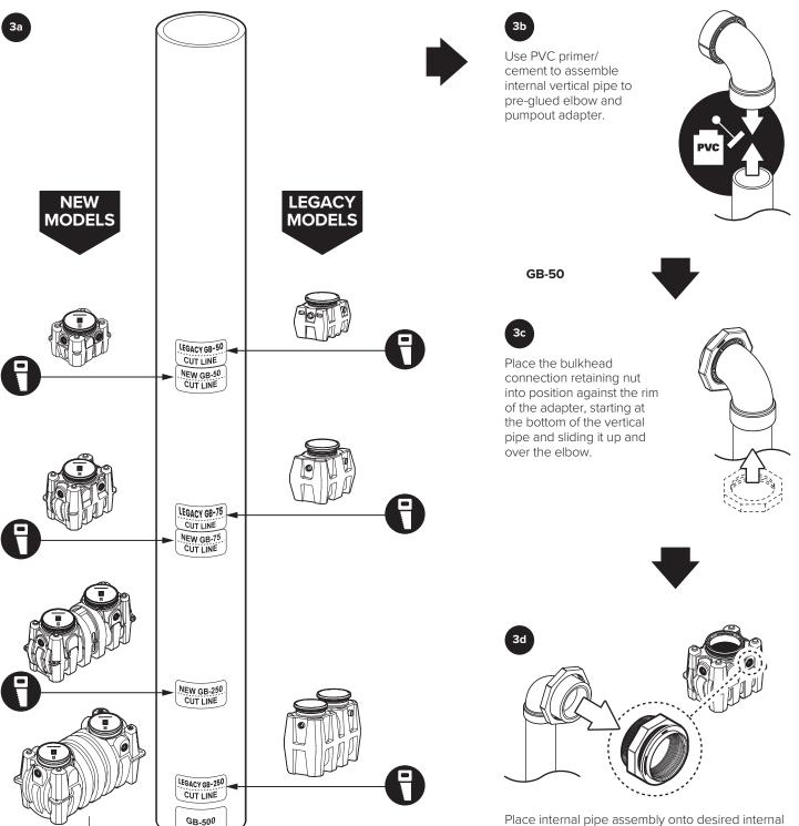
For new or legacy GB-50, GB-75 or GB-250, cut internal pipe at pre-labeled location and keep the top section. For GB-500 use entire length of supplied pipe.
