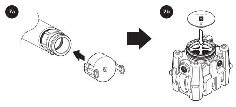
Install cam and groove cap at hookup
