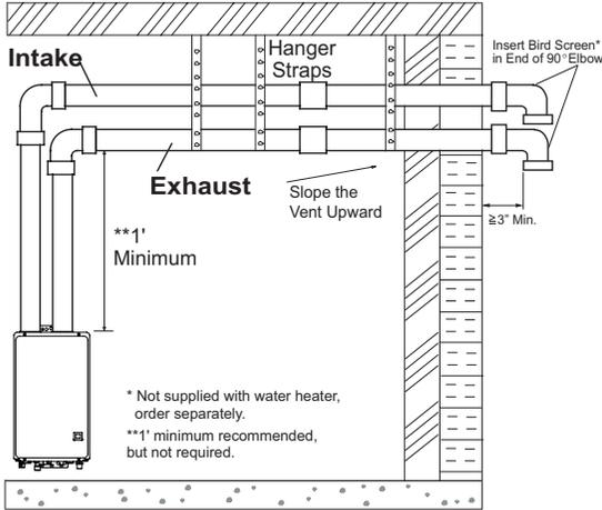
When choosing intake and exhaust terminations, you must use the same type of elbow (i.e. both 90° elbows). This will help with proper combustion by putting both terminations in the same pressure zone.
