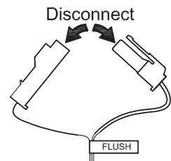
The gas water heater can not operate if the "blue connector" for flushing is connected.
