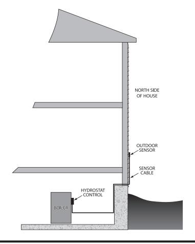
Before installation, determine the proper location for the sensor
