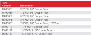
Can also be used with PEX piping. For PEX pipe sizes, refer to the Copper Tube Size column. Clip must be installed with temperature at or above 14 °F (-10 °C).
