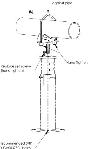
Accepts 1/2" fastener for recommended 3/8" DROP-IN-ANCHOR CADDY CA0037EG. Holes can be drilled out to accept larger fasteners.
