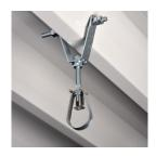
The 115M Standard Duty Loop Hanger is ideal for suspending stationary, non-insulated pipe lines, including CPVC pipes, in fire sprinkler systems. A knurled insert nut helps simplify vertical adjustments and flared edges on the base (1/2" to 4" sizes) help protect pipes from coming into contact with any sharp edges of the hanger.
