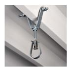
The 115M Standard Duty Loop Hanger is ideal for suspending stationary, non-insulated pipe lines, including CPVC pipes, in fire sprinkler systems. A knurled insert nut helps simplify ver 1150800EG and flared edges on the base (1/2" to 4" sizes) help protect pipes from coming into contact with any sharp edges or the manger.
