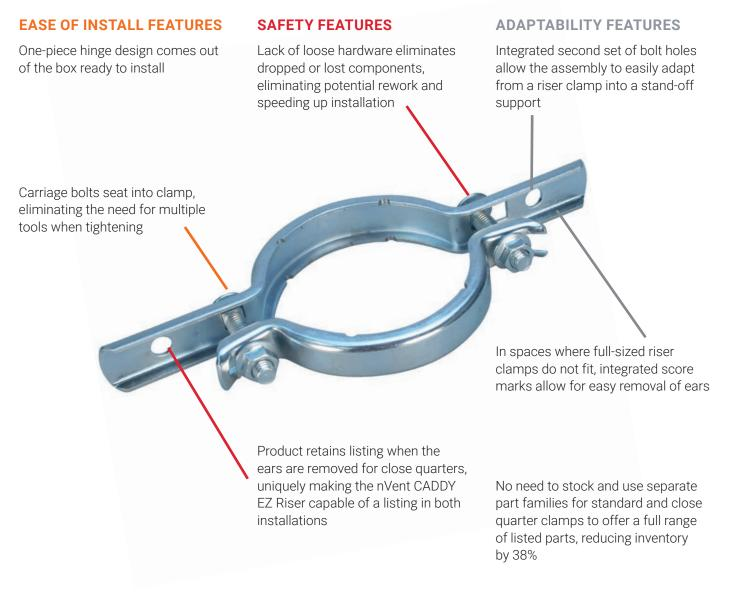
Conforms with Federal Specification WW-H-171 (Type 8), Manufacturers Standardization Society (MSS) SP-58 (Type 8)
