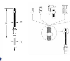
Material: Steel Finish: Electrogalvanized Static Load Safety Factor: 3.5:1
