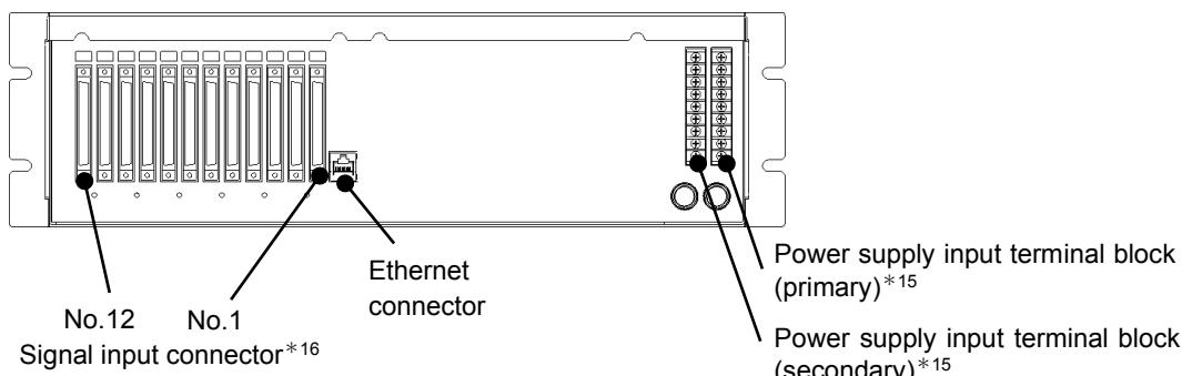
\*15 The unit has terminal blocks at both ends, even when code "0 (not available)" is specified for secondary power supply; however, the terminal block for secondary power supply cannot be used. Also, do not use the terminal block for other purposes including signal relay, etc.
