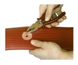
2a) The size of the repair patch should be 2 mm smaller than the removed external cover.
