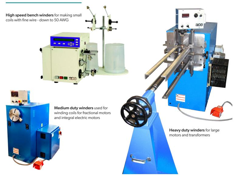
Coil winding accessories, such as winding heads, tailstocks, de-reelers, wire racks, and tension devices, are all part of the ACE/Benko product line. We provide everything you need to wind perfect coils!
