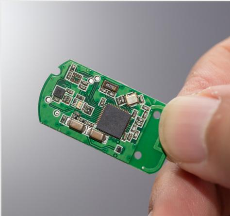
Finger print oils and salts must be removed prior to conformal coating.
