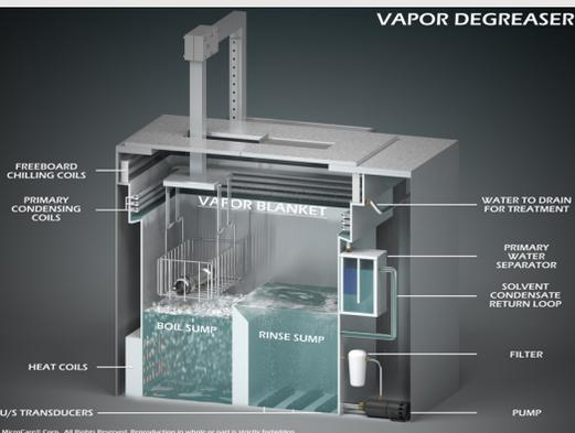
*Vapor degreasing cleans and dries PCBs in one step.*
