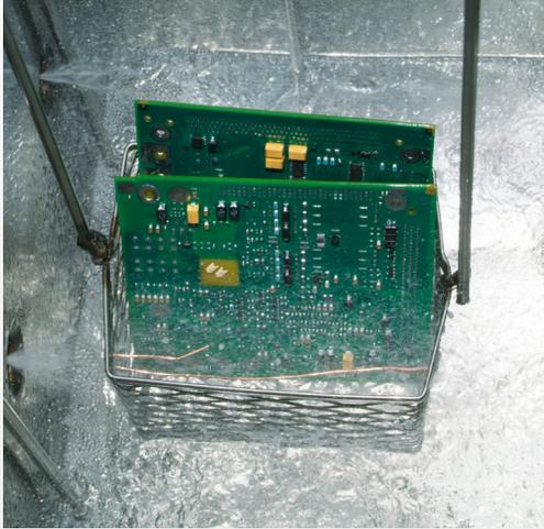
Vapor degreasing uses cleaning fluid immersion, combined with vapor rinsing and drying to remove contamination.
