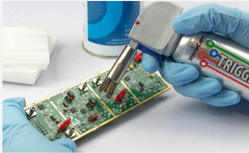
*The four steps to successfully cleaning PCBs are wet, scrub, rinse and dry.*
