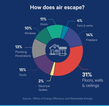
Nearly **one third** of air infiltrates through the openings in ceilings, walls and floors in a home with fiberglass insulation.
