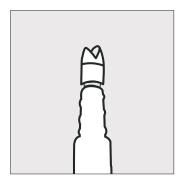
Nozzles provided allow for a fan spray pattern.
