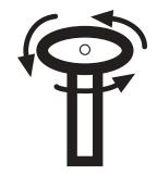
Open the valves completely by turning the valves COUNTER CLOCKWISE. Cylinder valves must be upright during use.
