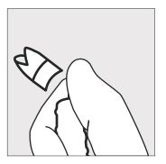
Snap-tip nozzle now allows for a cone spray pattern.
