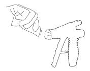
Change nozzles frequently! Foam will cure inside the nozzle in the same amount of time that foam becomes tackfree in the air.
