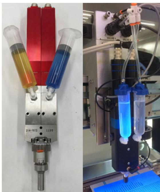
2K coating materials can be applied thinly (50-75 $\mu$ m), however they have been designed, formulated and tested to be applied at much greater thicknesses (250-300 $\mu$ m), to facilitate superior encapsulation of components and component leads.
