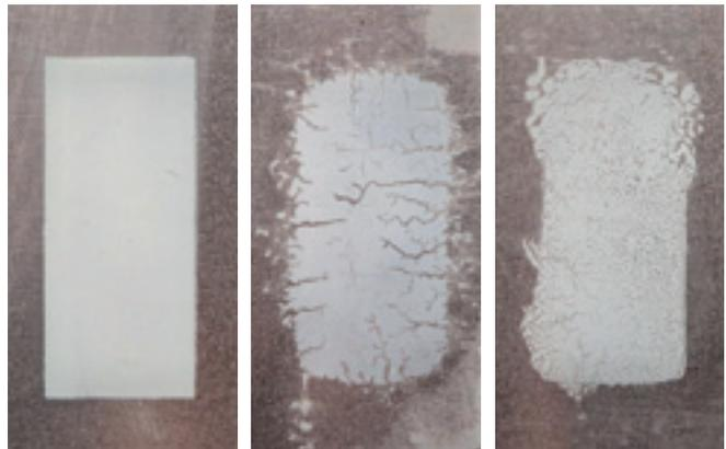
Photographs illustrating the difference in performance following thermal shock testing between  $-40^{\circ}\text{C}$  and  $+125^{\circ}\text{C}$ .
