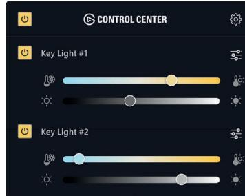
Use Control Center to switch Key Light on/off, adjust brightness, and fine-tune color temperature.
