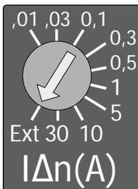
In switch position "Ext", the values can be changed via the Modbus RTU interface.
