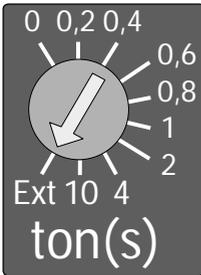
The residual operating current and the pre-warning must be exceeded at least for the set response delay  $t_{on}$  to trigger the respective alarm. The amount by which the response value is exceeded is not relevant.
