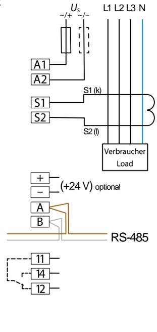
Abb. 3-3 Wiring diagrams RCM410R-1 and RCM410R-2
