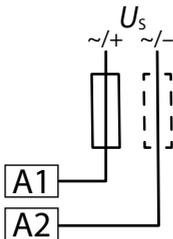
The RCM410R-2 can be alternatively operated via terminals A1 and A2 with a voltage of AC/DC 100...240 V. In this case, the device must be provided with a back-up fuse. The connection is made at the top side of the device.
