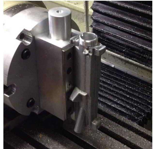
MILLING BARREL THREAD ON 4 TH AXIS FIXTURE
