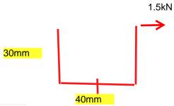
Plate thickness is 2.5mm M=1.5kN\*30mm=45000N.mm Stress M/z=45000\*6/1000\*2.5\*2.5=43.2MPa
