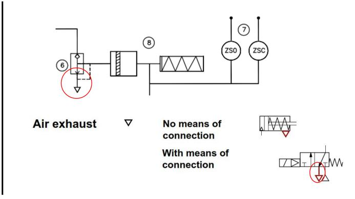
Triangle symbol should be interpret with the line attached or without? **Exhaust or Exhaust with means of connection (Threaded)?**
