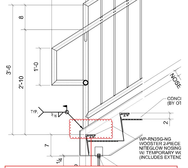
Channel flange is not of adequate width to allow for a 3/16" weld all around.
