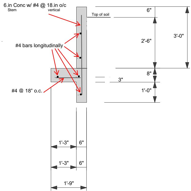
Detail for walls retaining 30" of soil at driveway and bridge areas
