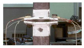
Figure 8.4 - Tension test of a flange-plate joint bolted along two RHS sides, showing plate flexure
