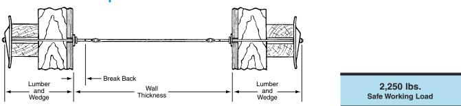
Dayton Superior A-3 Standard Snap Ties are manufactured with either hot or cold forged integral heads. A-3 snap ties have a nominal 1" breakback with 1/4" and 1/2" breakbacks available on special order. Breakbacks over 1" can be provided on special order, but due to the increased concrete bond Dayton Superior cannot guarantee that the ties will consistently provide proper breakback. Coating the tie ends with wax will aid in breakback operation.
